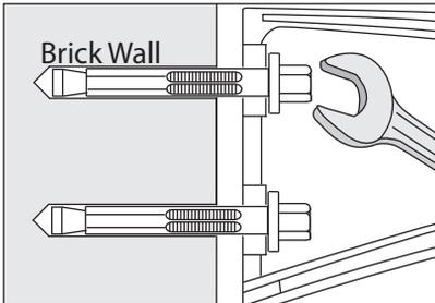
3. Expand anchor by tightening nut or head 2 to 3 turns.
