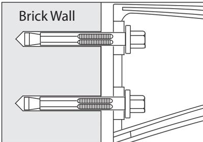
2. Insert assembled anchor into hole, so that washer or head is flush with materials to be fastened. \*DO NOT unscrew the head. Insert it as is. If it is stiff, use rubber hammer to insert.
